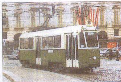
Car 3501 was unique in the ATM fleet, having been reconstructed in the undertaking's own workshops from war-damaged Fiat bogie car 3001. It was not heavily rebuilt in 1976/77 in the manner of the main batch of post-war cars and retained a single centre doorway. Now preserved, it enters Piazza Castello on 2 December.
