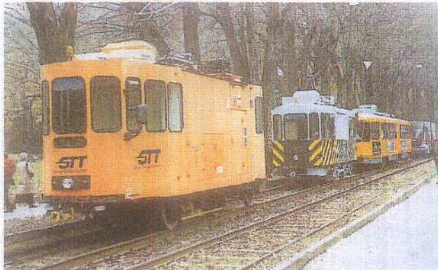
Several current Torino works cars were on display in Viale Primo Maggio. Rail-scrubber T420 has a new body which renders it unrecognisable from its former state. Behind is Sabbiera (sand car) T427, fitted with a new metal body in 1989; whilst six-axle articulated car 2877, rebuilt in 1982 from a pair of large Peter Witt pre-war bogie cars, is in the rear.
