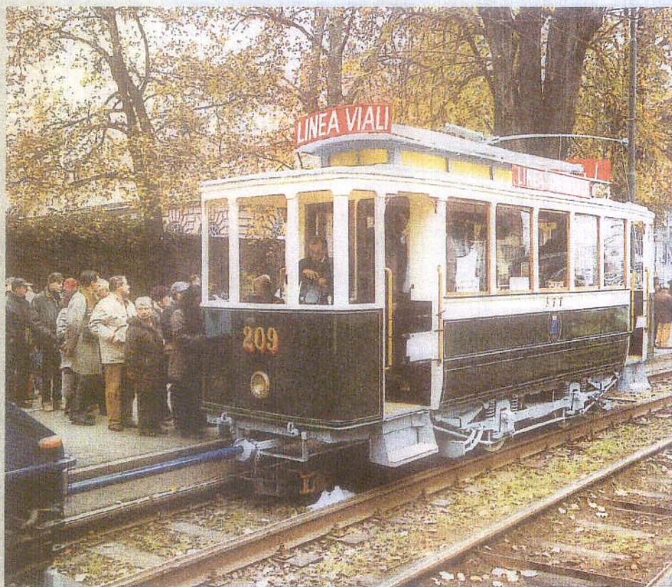
Trams don't need to be new, or even have seats, for people to be queuing up to get on them! The first renovation job by Torino's recently-formed ATTS is of former works car T426, now restored to its 1911 state. The interior has yet to be fitted out and the car lacks electrical equipment. It was displayed on Viale Primo Maggio, where queues formed to inspect the model tramway layout on display inside. Mike Russell
